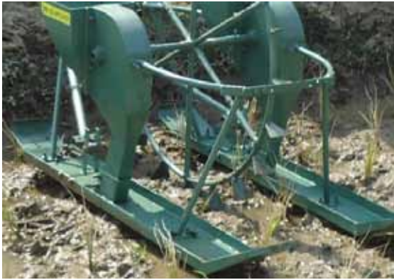
Fig. 1. Adjusting mechanism of the applicator with line spacing.
