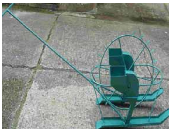
Fig. 2. BRRRI USG applicator.
