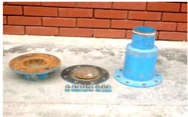
Fig. 2. Different components of the check valve with threaded fittings
