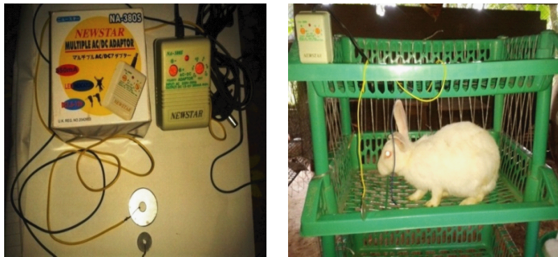
Fig. 1: (a) Electro-stimulation device with two electrodes (b) Plastic shelf-rack with rabbit in electrotherapy chamber.
