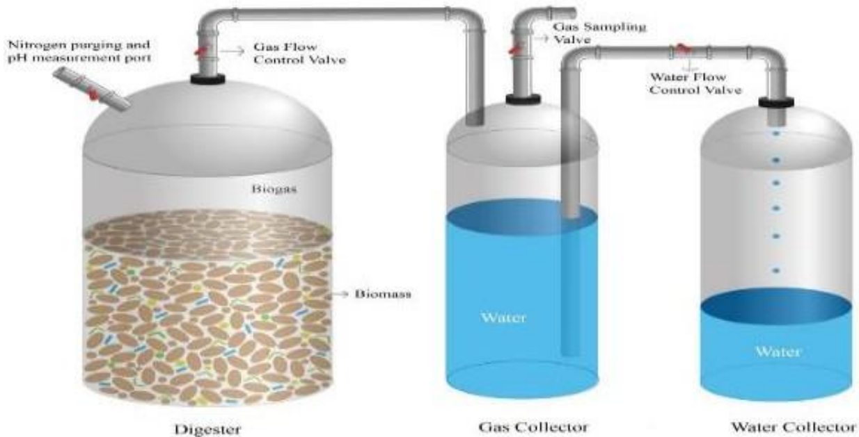
Figure 1: Process flow diagram of dry anaerobic digestion process (Hossain et al., 2022)
