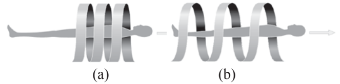
Fig 9: (a) Pitch is low; (b) Pitch is high Images in 3 planes after reconstruction:
