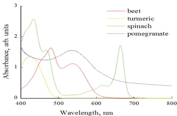
**Fig. 2:** UV-vis absorption spectra of beetroot, turmeric, spinach, and pomegranate extracted dyes
