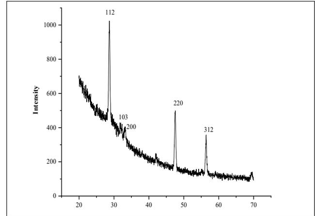
**Fig. 4.** The XRD patterns of the sulfurized CZTS thin films prepared from the chloride chemical based precursor.
