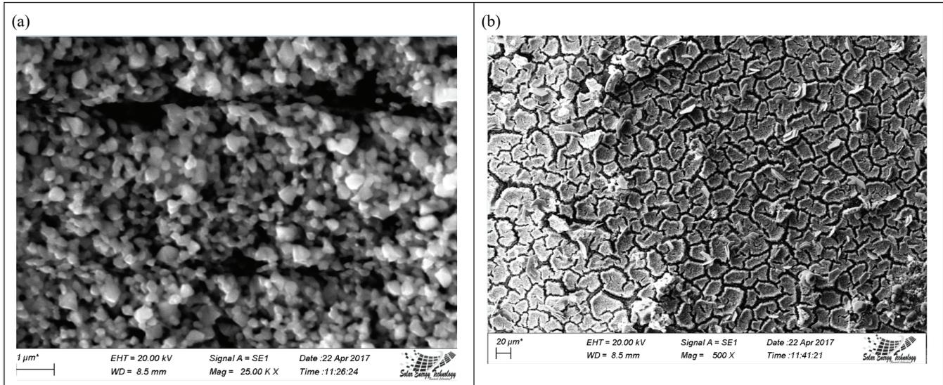
**Fig. 5.** The surface morphology of the CZTS thin film [(a) 25000X (b) 500X].
