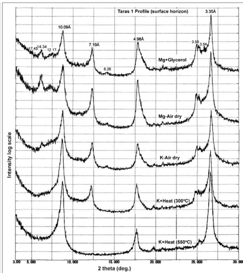
Fig. 4. X-ray diffractograms of clay sample of Taras 1 soil.
