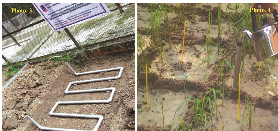
Photographs 3-4. Instrument and approaches for the elevation of soil temperature rise of 2 and 3°C during field study.
