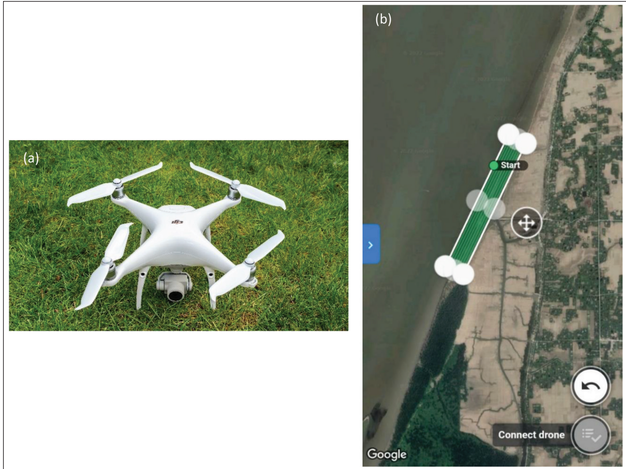
Figure 2: The Image (a) is a Photograph of the DJI Phantom 4 Pro V2.0 Drone. The Drone has a 20MP Camera and 1” CMOS Sensor which Captures RGB Images. The Image (b) Shows a Representative Flight Plan along the Intertidal Zone of Manpura Island
