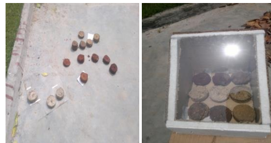
Fig. 3. Drying briquette (a) under sun (b) using a solar dryer
