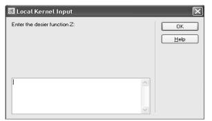
Enter the desire function Z:  $3x_1 + 5x_2 + 2x_3$ ; Then, n = 5; Enter Row 1: 1, 2, 2, 1, and 0 Enter Row 2: 2, 4, 3, 0, and 1 Enter co-eff. of objective function: 3, 5, 2, 0, and 0 Enter upper bound: 4, 3, 3, 9999, and 9999. Enter co-eff. of basis element: 0, 0 Enter constant: 10, 15  $X_1 = 0$ ;  $X_2 = 0$ ;  $X_3 = 0$ ;  $X_4 = 0$ ;  $X_5 = 0$ The initial simplex table is generated by the following codes.
