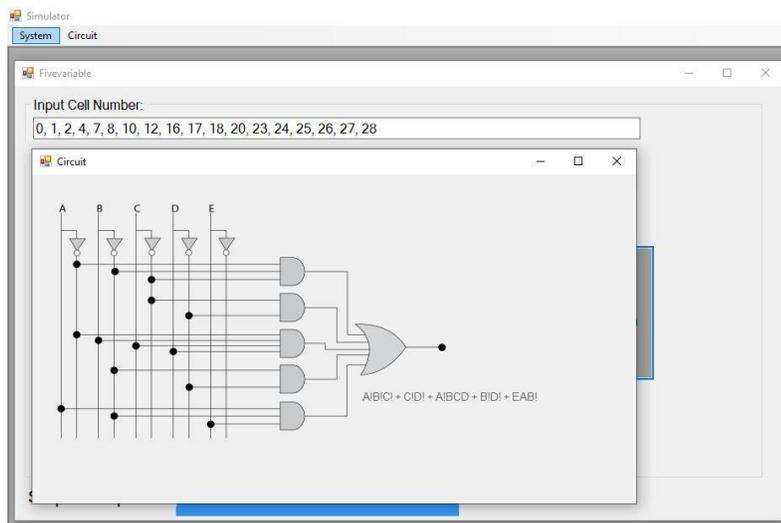
Fig. 10: The Circuit Diagram for the 5 Variables
