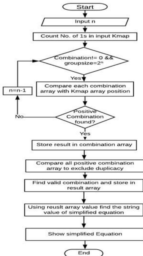
Fig. 3: System Flow Diagram for the K-Map
