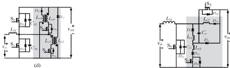
Fig. 6. Switched inductor network (a) with diode [58] (b) in coupled formation (c) in LC formation [25] (d) in double coupled formation [39]
