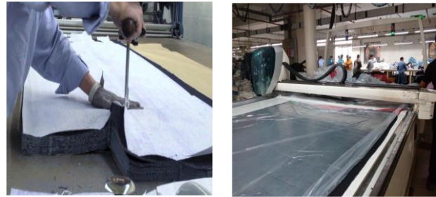
Fig.2. Straight knife fabric cutting and Semi automatic fabric spreading machine
