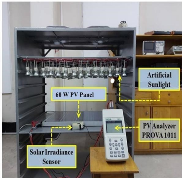
Fig 2. Experimental setup of a 4×4 PV array for testing different interconnection topologies at the non-uniform aging condition.
