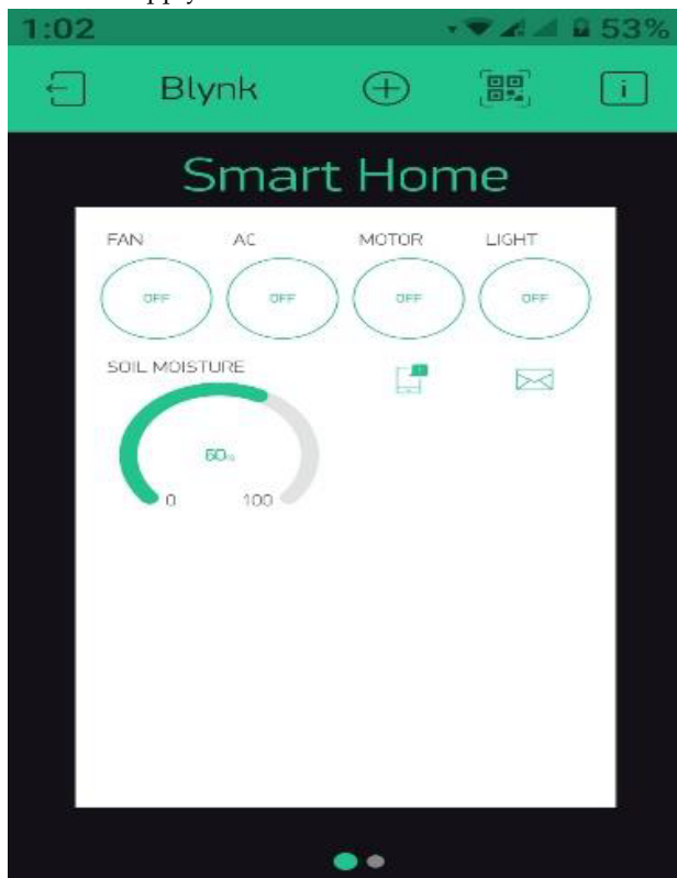
(b) Measurement of the soil moisture and motor turn on/off in apps
