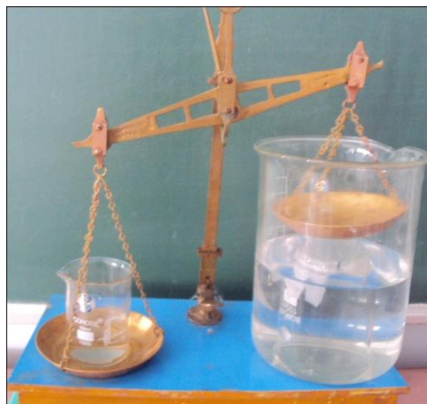
Figure 4: Modified two arm balance used for bioadhesive test (detachment of pan from the membrane on the addition of water to the other pan).
