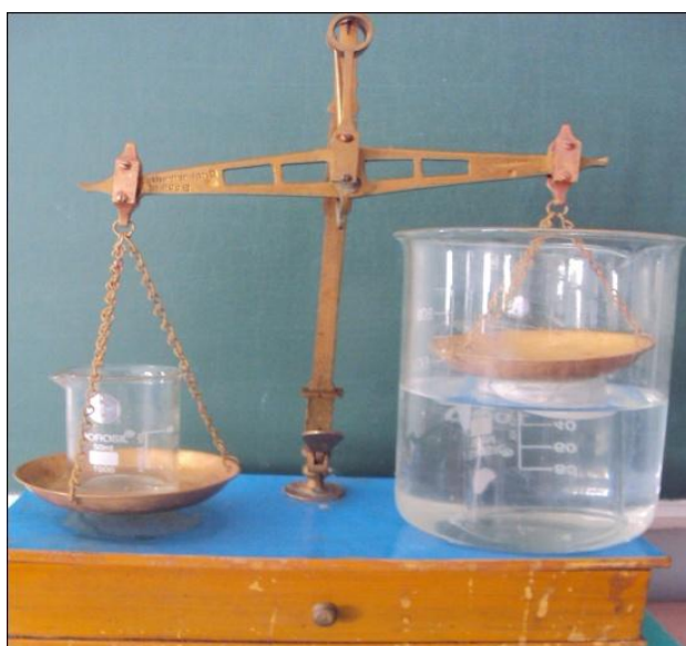
Figure 3: Modified two arm balance used for bioadhesive test (preload was put on modified arm for attachment of gel to the biological membrane).
