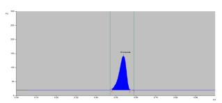
Figure 2: Densitogram of standard gliclazide (800 ng/spot); peak 1 (RF: 0.58). toluene: ethyl acetate (1.0: 1.0, v/v).
