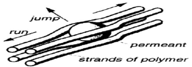
Figure 4: The jump-and-run model of permeant diffusion through intact polymer.
