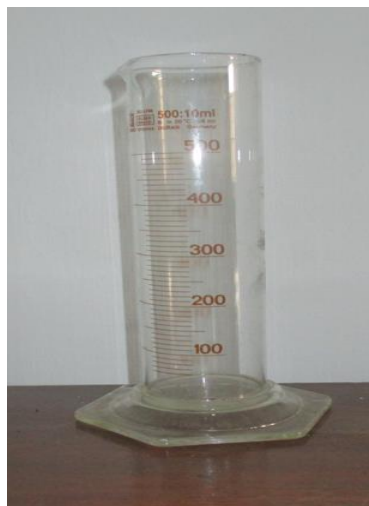
Figure 6. Graduated 500 ml Measuring Cylinder for Measuring Paddy Bulk Volume.
