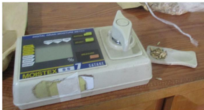
Figure 2. Moisture Meter for Measuring Paddy Rice Moisture Content.
