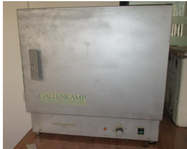
Figure 4. Bench Top Laboratory Oven for Drying Paddy Rice.
