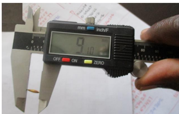
Figure 3. Vernier Calliper for Measuring the Axial Dimensions of the Paddy Rice.
