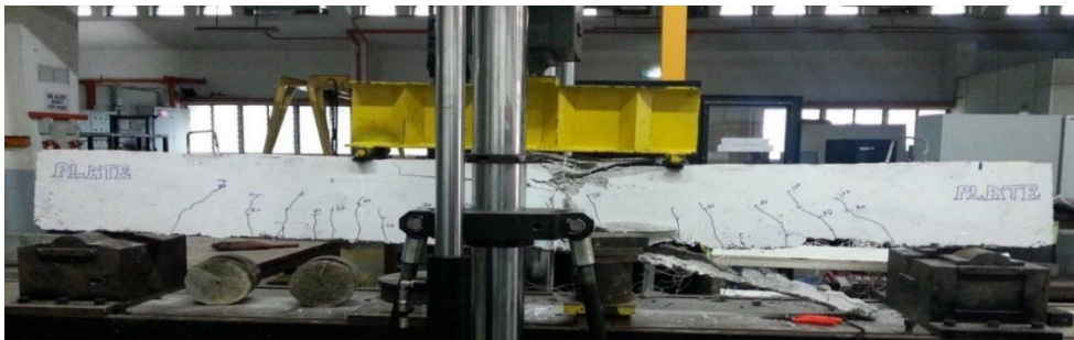
Figure 1: Instrumentation setup for flexural performance investigation
