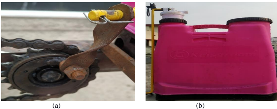
Figure 2: (a) Crank mechanism connected with short sprocket and connecting rod, and (b) Knapsack sprayer
