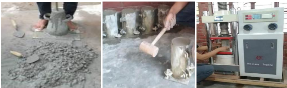
Figure 3: Sample preparation and test set up for compressive strength test
