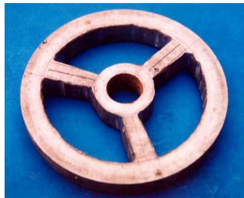
Fig. 6. Follower piston plate made with moulded cast iron disc for piston valve type-II, III and IV
