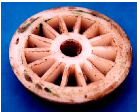
Fig. 5. Follower piston plate and check plate made with plastic disc for piston valve type-I and check valve type-I
