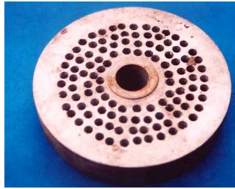
Fig. 4. Piston plate made with perforated cast iron disc of slots size 6 mm for piston valve type-IV
