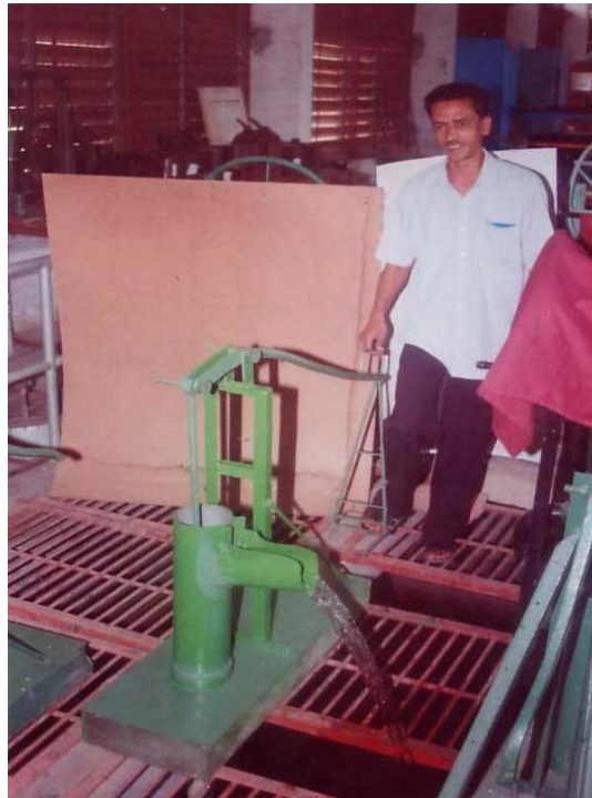
Fig. 11. A photographic view of the pedal pump and its operation
