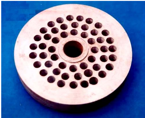
Fig. 3. Piston plate made with perforated cast iron disc of slots size 8 mm for piston valve type-III
