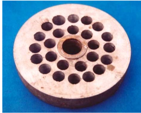
Fig. 2. Piston plate made with perforated cast iron disc of slots size 11 mm for piston valve type-II
