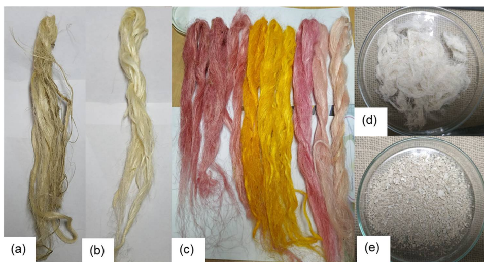
Fig. 2. Preliminary observation of STLF and products. (a) Untreated fibres, (b) bleached fibres, (c) dyed fibres, (d) cellulose and (e) crude microcrystalline cellulose.
