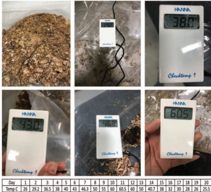
Figure 1. A compost heap of 1 m length *1 m width *90 cm height, was made from SPF broilers' litter and sawdust, the digital thermohygrometer was used to monitor temperature for 20 days.
