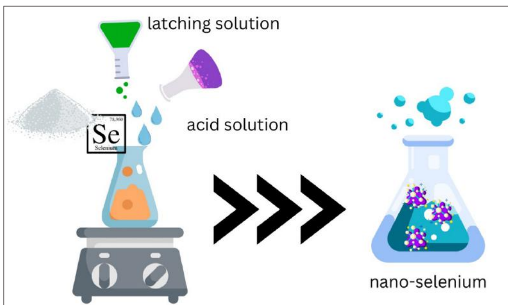
Figure 4. The chemicals method produced nanomaterials (adapted from Aguilar [63]). The principle of making nano selenium chemically is basically by utilizing a low pH solution at a high temperature to rupture mineral bonds so that nanosize is formed, in addition, anti-aggregation substance is also added so that nano selenium granules are expected not to reassemble.
