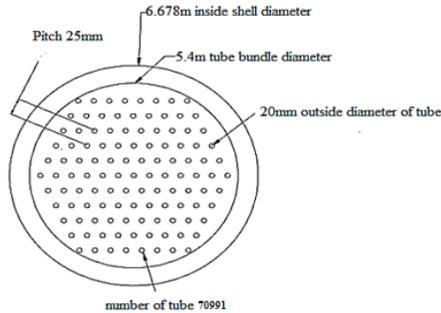
**Fig. 9.** Suggested condenser's physical parameters for triangular tube bundle arrangements and a shell.
