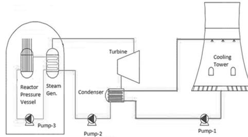
**Fig. 1.** Nuclear Power Plant Cycle
