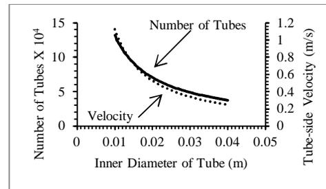
**Fig. 2.** Velocity of fluid inside a tube vs. inside diameter of a tube and number of tubes of a condenser vs. inside diameter of a tube for a constant tube length of 14 m.
