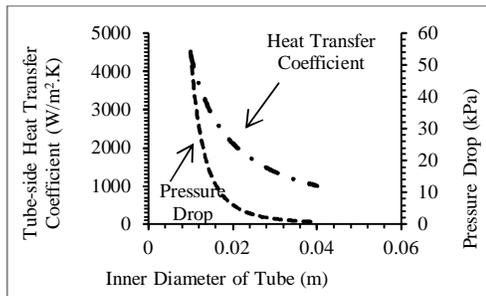
**Fig. 3.** Heat transfer coefficient inside the tube vs. inside diameter of a tube and pressure drop inside A tube fluid vs. inside diameter of tube for a constant tube length.
