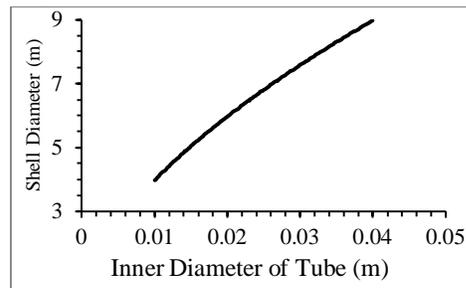
**Fig. 5.** Diameter of a shell of a condenser vs. outside diameter of tube for a constant tube length.
