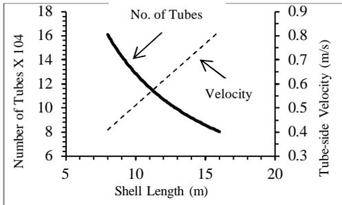
**Fig. 6.** Velocity of fluid inside a tube vs. length of a tube and number of tubes vs. length of a tube for a constant inside diameter of a tube.
