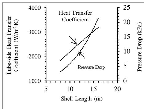
**Fig. 7.** Heat transfer coefficient inside a tube vs. length of the tube and pressure drop inside a tube vs. length of the tube for constant inside diameter.
