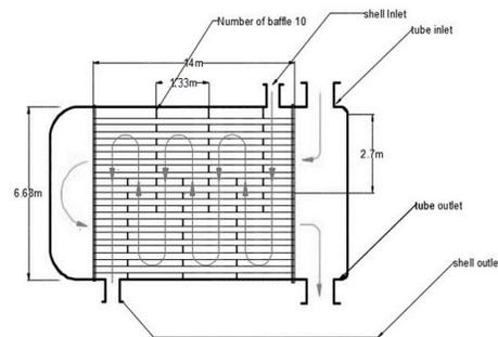
**Fig. 8.** Suggested design of a shell and tube condenser.
