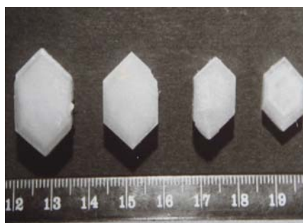
Fig.2. Photograph showing some of the grown thiourea crystals.
