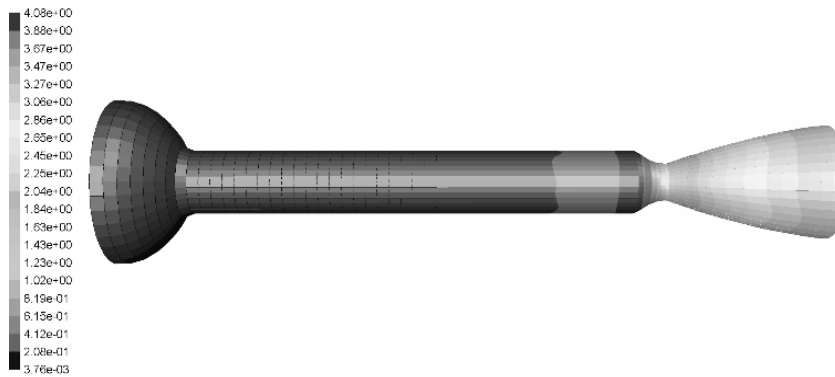
Fig. 6: Mach number distribution across the wall.
