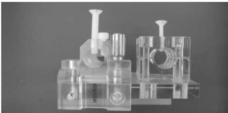
Fig. 2. Special holder for the special chambers used in the PDD measurement.
