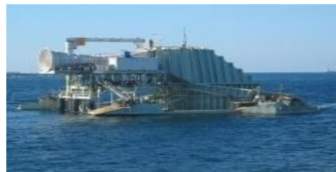
Image of oscillating water column
