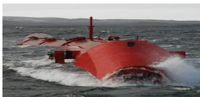
Image of surface attenuator
