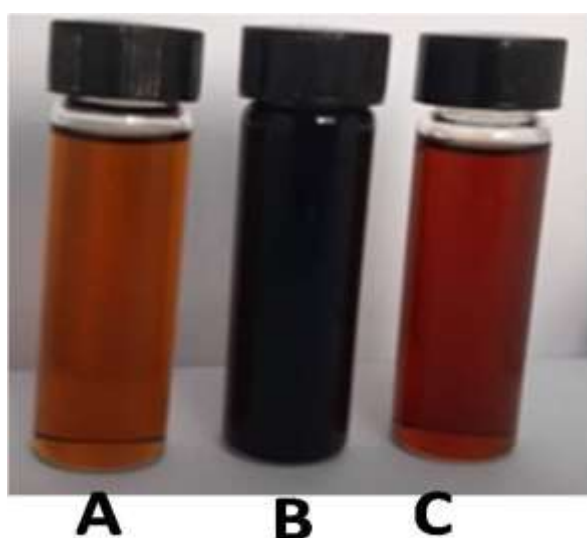
Fig. 4. Picture of engine oil purified by clay/activated charcoal(A), waste engine oil(B), and engine oil purified by acid-treated clay (C).
