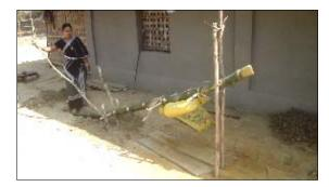
Fig. 9. Paddle-operated polishing method
