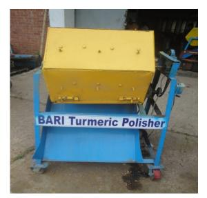
Fig. 3. The pictorial view of the turmeric polisher
