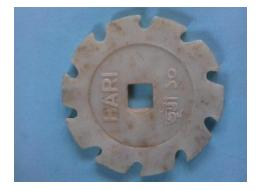
Fig. 5. Seed metering device
