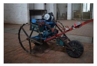
Fig. 2. Motor operated seeder
