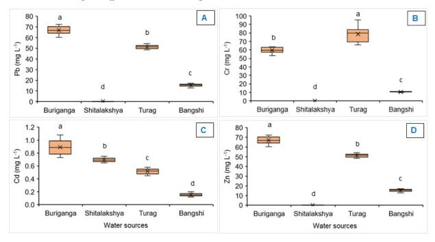
Fig. 2. Boxplot of the concentration of heavy metals (Pb, Cr, Cd and Zn) of different river-water of Dhaka city. Median values are denoted by solid lines within the box while box boundaries show the 1<sup>st</sup> and 3<sup>rd</sup> quartiles. Box whiskers indicate the highest and lowest data values. Boxes with similar letters are statistically similar at 5% level using Tukey's method and vice versa.
