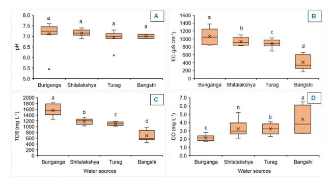
Fig. 1. Boxplot of pH, EC, TDS and DO concentrations of different river-water of Dhaka city. Median values are denoted by solid lines within the box while box boundaries show the 1<sup>st</sup> and 3<sup>rd</sup> quartiles. Box whiskers indicate the highest and lowest data values. Boxes with similar letters are statistically similar at 5% level using Tukey's method and vice versa.
