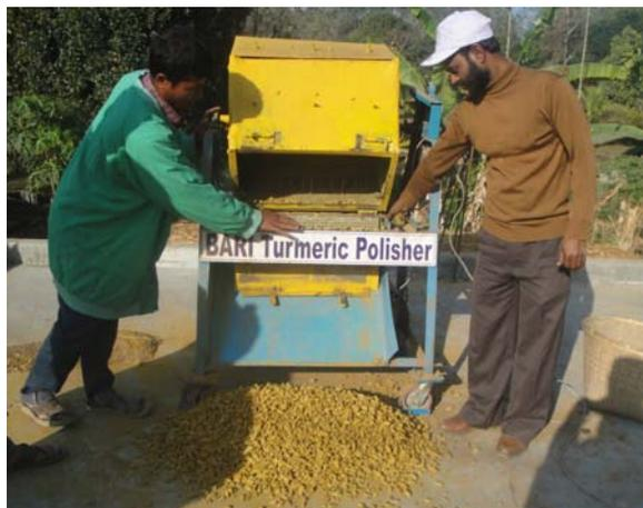
Fig. 6. Discharging of turmeric from the polisher
