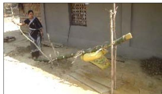
Fig. 9. Paddle-operated polishing method
