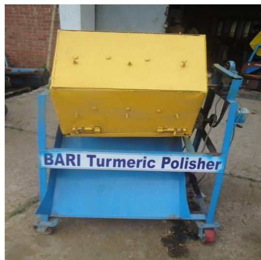
Fig. 3. The pictorial view of the turmeric polisher
