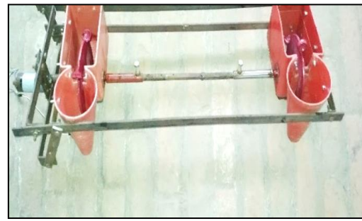
(b) Modified granular urea applicator structure
