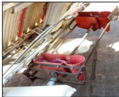
(a) Granular urea applicator attachment with rice transplanter
