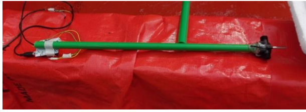
Fig. 4 Temperature and Flow Sensor with Microcontroller
