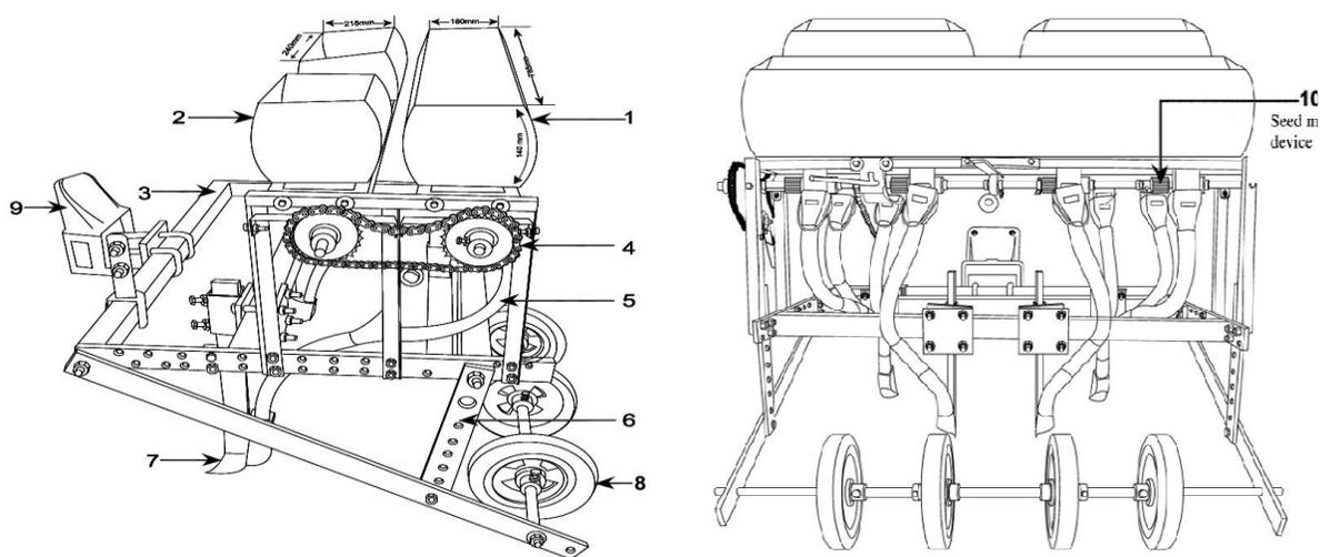
1. Seedbox, 2. Fertilizer box, 3. Toolbar frame, 4. Chain and sprocket, 5. Seed tube, 6. A depth control device, 7. Furrow opener, 8. Press wheel, 9. Hitch plate, 10. Seed metering device
