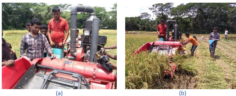
Figure 3. GPS receiver recorded data during mini combine harvester operation. (a) Installing GPS receiver on mini combine harvester, (b) Harvesting paddy with mini combine harvester
