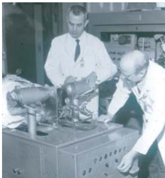
Fig.-4: First clinical positron imaging device
