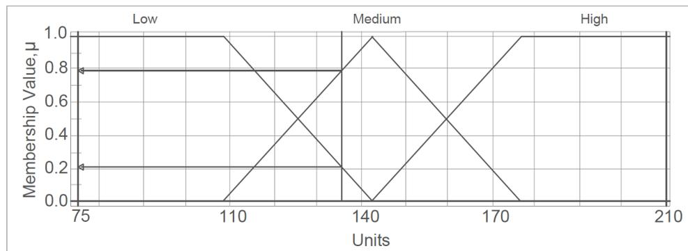
Fig. 2: Membership function for 'Travel Time' input variables
