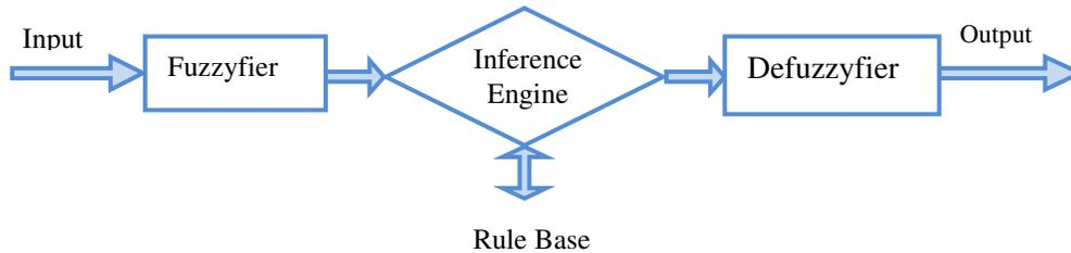
Fig. 1: Block Diagram of Fuzzy inference systems
