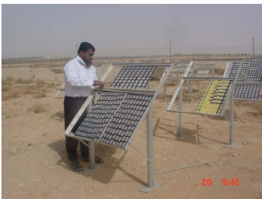
Fig.1. Exposing plastic samples in natural weathering condition. Films are fixed on plexy glasses and oriented in a steel rack at 45 degree angle with the basement and facing to east so that maximum amount of sunlight fall on the film in all time.
