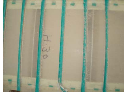
Fig.2. Photographs of sample containing 50 percent Polystarch-plus-H additive. It was taken after 9 months which shows that all the exposed parts were severely degraded and were taken away by air. Only small amount of sample which are attached by the tapes are left.
