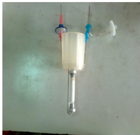
Fig 1 : Tc-99m generator Column fixed with needles
