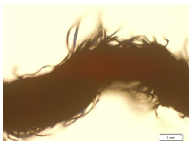
Fig. 4: FM image of stone-bleach treated warp yarn
