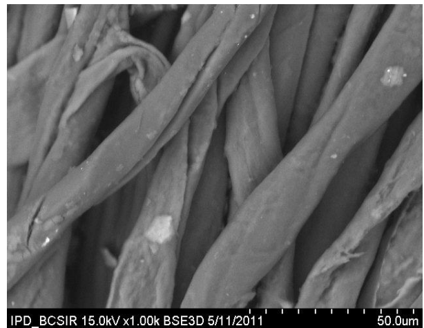
Fig. 2: SEM image of stone-bleach treated denim fabric
