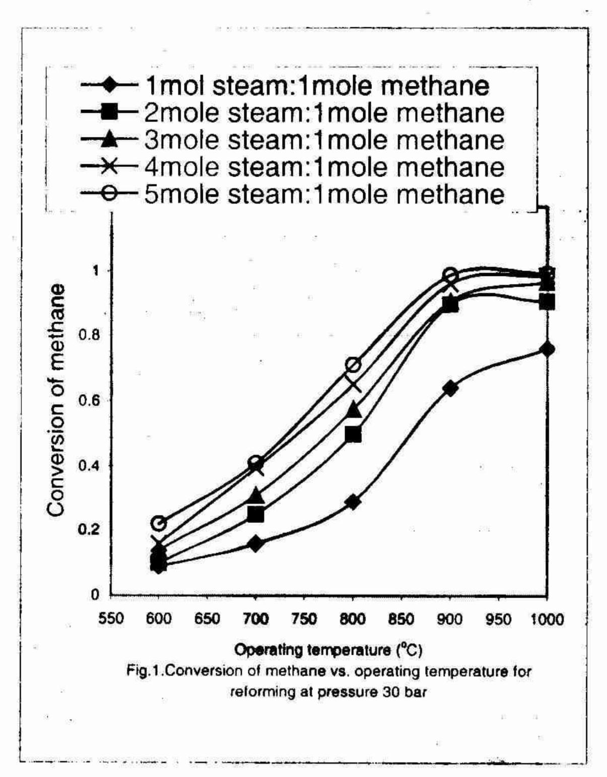
The same effect has been observed at pressure 10 and 20 bar 8. So at constant pressure and constant steam/methane ratio, the conversion of methane increases with the increase of temperature. On decreasing temperature, the effect is reversed. If low temperature is selected for any reforming system, other variables such as pressure should be decreased or steam/methane ratio should be increased for higher conversion of methane.
