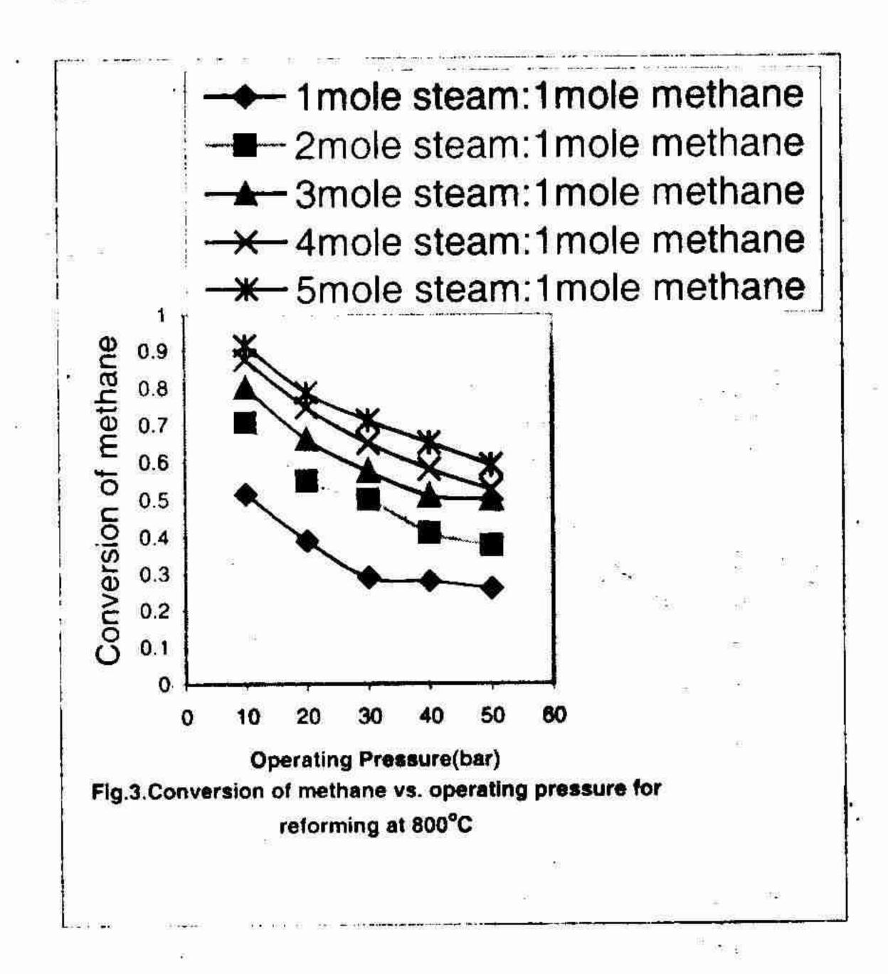
When pressure of 10 bar is applied for 50% conversion operating temperature should be 725°C. If 20 bar, 30 bar, 40 bar and 60 bar pressures are applied, temperatures should be 760°C, 793°C, 820°C and 855°C respectively for the same conversion of methane in steam reforming. For 60% conversion of methane operating pressure can be selected as 10 bar, 20 bar, 30 bar, 40 bar and 60 bar; but operating temperature should be 760°C, 810°C, 845°C, 875°C and 910°C respectively.
