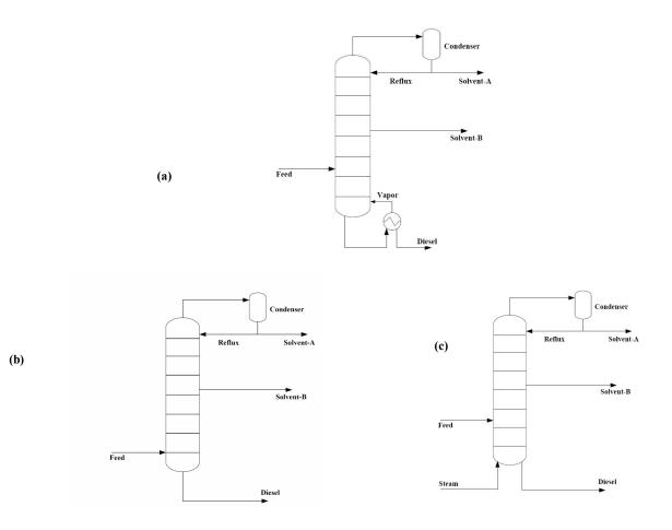
Fig 2. Design variations of the fractionation column – (a) Column-1, (b) Column-2, (c) 67 Column-3
