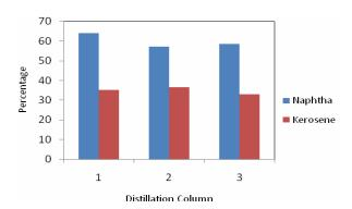
Fig 4(b). The percentage of Naphtha and kerosene in Solvent–B for three distillation columns
