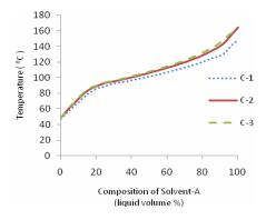
Fig 3(a). ASTM D86 data for Solvent-A obtained from the three different design consideration
