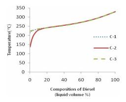
Fig 3(c). ASTM D86 data for Diesel obtained from the three different design consideration
