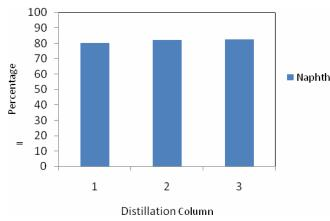
Fig 4(a). The percentage of Naphtha in Solvent–A for three distillation columns.
