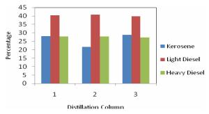
Fig. 4(c). The percentage of Kerosene, Light diesel and Heavy diesel in Diesel for three distillation columns
