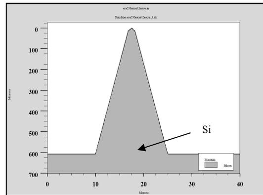
d. 600  $\mu\text{m}$  tall beveled Si microneedle, aspect ratio is 40:1
