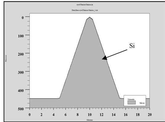
b. 450  $\mu\text{m}$  tall beveled Si microneedle, aspect ratio is approximately 50:1
