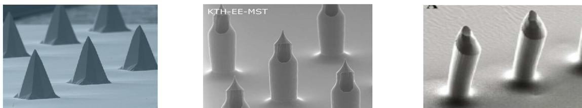
Fig. 1. Scanning Electron Microscopic (SEM) images of different types of microneedles.
