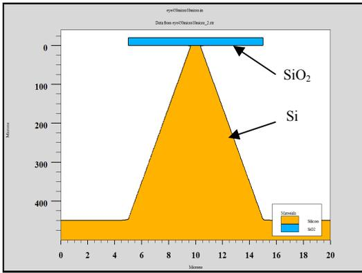
a. Si microneedle with etch mask ( $\text{SiO}_2$ ) shown after a complete RIE process
