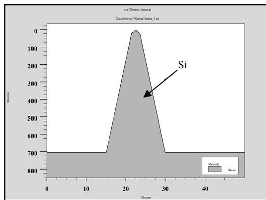
e. 700  $\mu\text{m}$  tall beveled Si microneedle, aspect ratio is approximately 46:1
