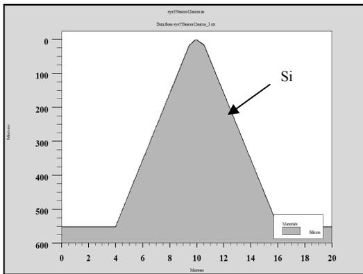
c. 550  $\mu\text{m}$  tall beveled Si microneedle, aspect ratio is 55:1
